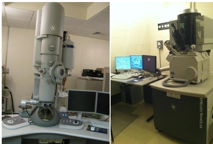
Figure 4.5. Transmission electron microscope (TEM) TECNAI F20 and Helios Nanolab 600 FIB/SEM. TEM left side and FIB right side, both equipments available at the Material research center (MRC) on the campus of Missouri S&T.
