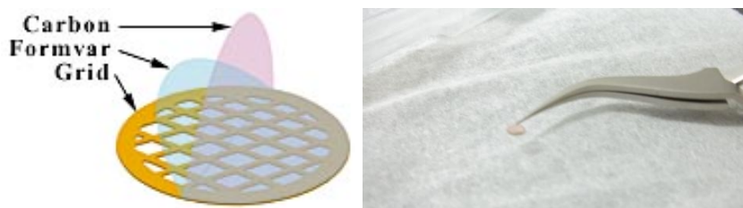
Figure 4.6. Schematic steps for sample preparation for STEM/TEM.
